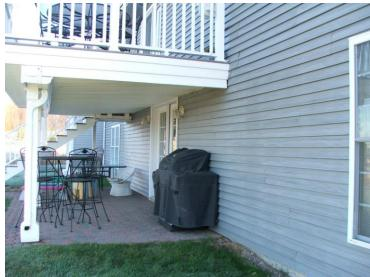
low maintenance material. A sample of doors were opened and operated freely. The deck(s) appear to be constructed from pressure treated wood – a rot resistant material. It appears that the surface of the rear deck is wood fiber/plastic composite, a water resistant material. The deck/porch railings are firm. The canvas awning opened and closed with ease. No holes or badly worn areas were noted.
